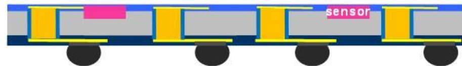
Active Interposer with die to die or die to wafer stacked sensors
